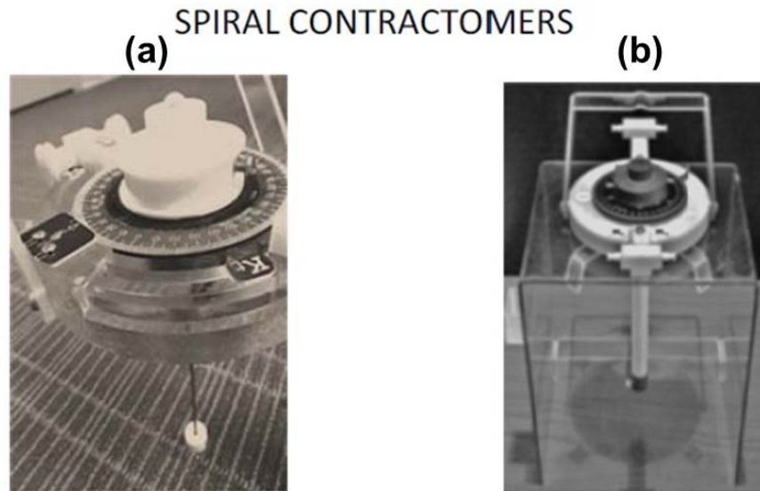
Figure 1 - Spiral contractometer designs: (a) Prior design; (b) New design.
